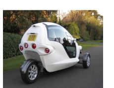
**Example EVs** The S.A.M. from Poland, left, offers compact dimensions and frugal energy consumption<sup>8</sup>, yet full weather protection and stability. The innovative Libner BIL delivery system from France, right, provides new solutions for urban freight distribution (800kg load capacity).
